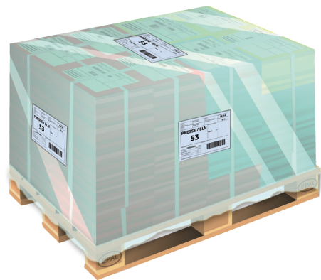
Fig. 30: Pallet labeling with three routing labels This example is for illustration only
